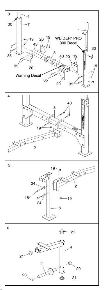
7. Lubricate an M10 x 72mm Bolt (40). Attach the Leg Lever (4) to the Front Leg (8) with the Bolt and an M10 Nylon Locknut (19).
